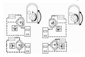
2. EUROMIX actuator with FMV 140 valve installation example.
